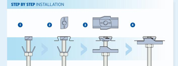
Pre-assemble the locking plate and wedge (flat surface facing up) onto the threaded rod.
